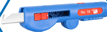
Quadro-Stripper multifunctional stripper, working range stripping 0,5 - 6,0 mm 2 / skinning 8 - 13 mm Ø
